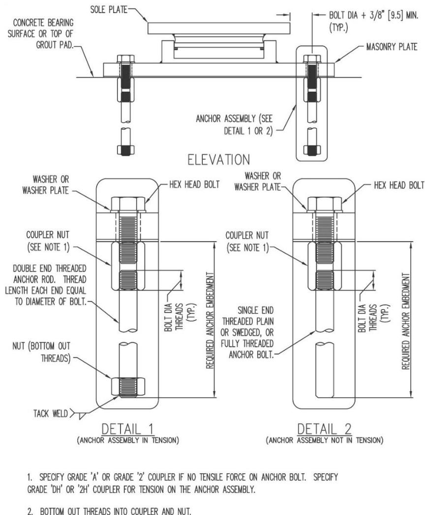
**Figure 5 Sketch of a removable bearing detail.**
