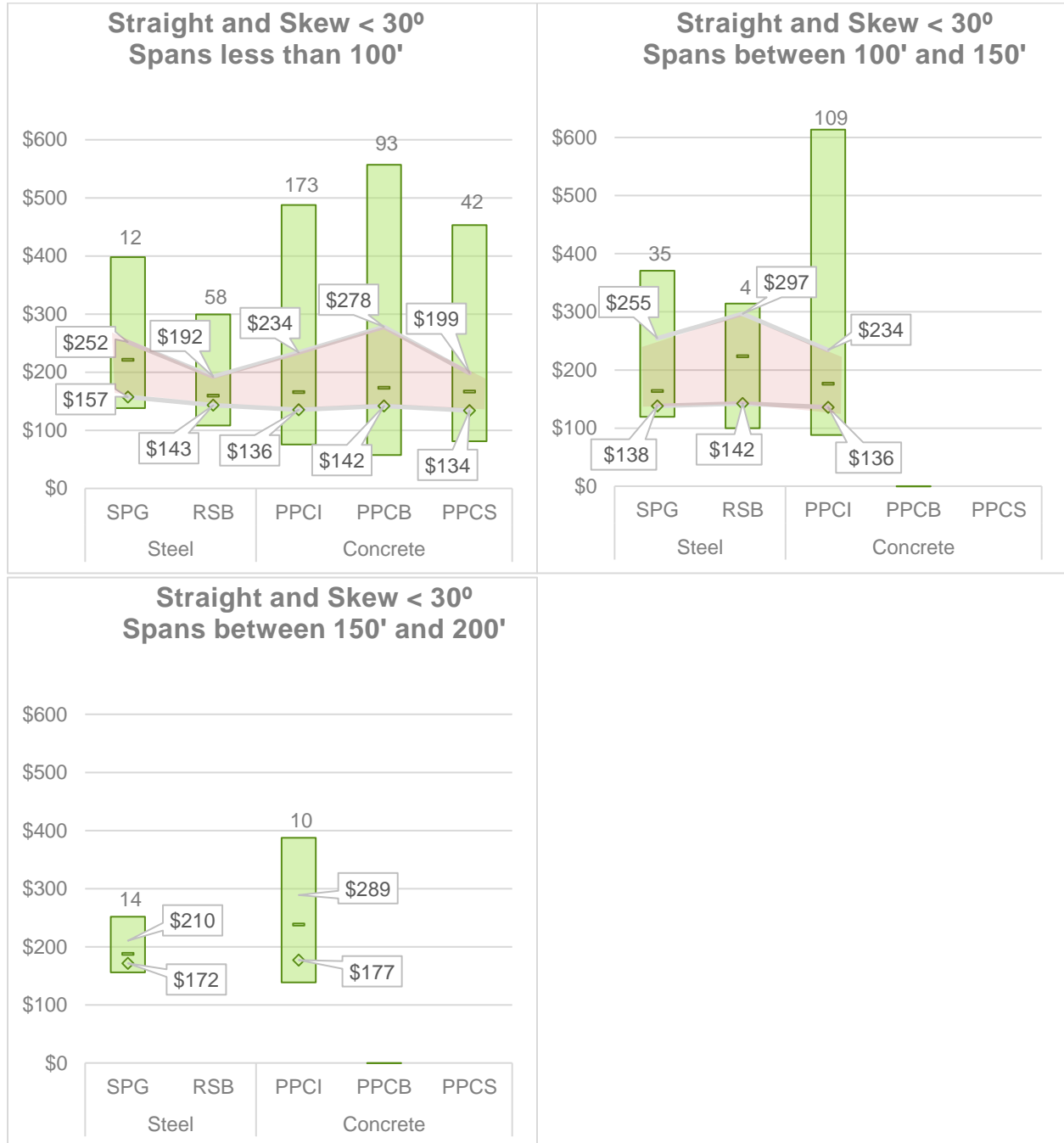
Figure 7: Average Cost by Span Length for Straight and Skew < 30° Bridges – National
