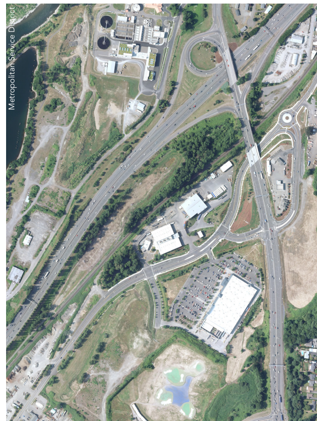
▲ An aerial view of the overall project site illustrates the reworked interchange, including the new roundabout and the new bridge to the west.
