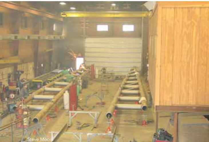
▲ The first stage of fabrication, with trusses positioned for ease of access and welding.
