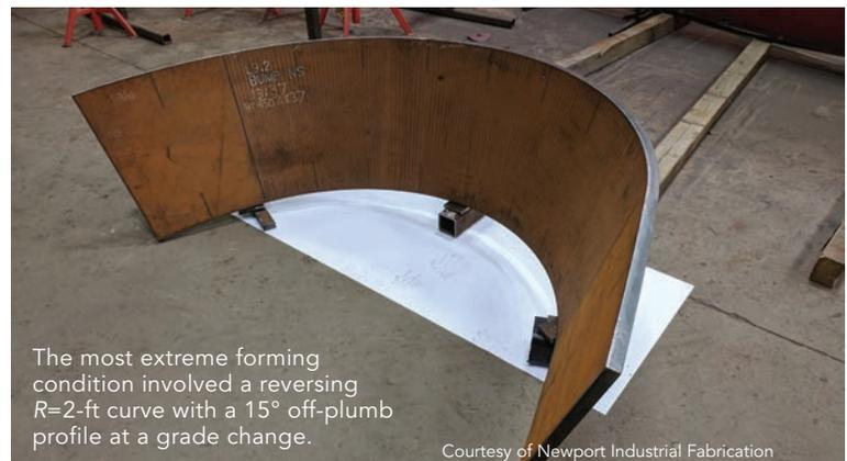
The most extreme forming condition involved a reversing R=2-ft curve with a 15° off-plumb profile at a grade change.
