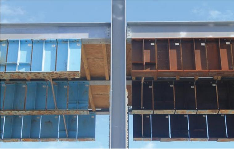
above: The first statistically significant probability of detection (POD) study for visual inspection of fatigue cracks was conducted at S-BRITE. Weathered painted specimens are shown on the left, and uncoated weathered specimens are on the right.
