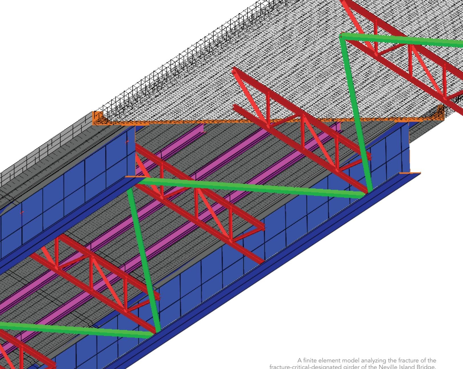
A finite element model analyzing the fracture of the fracture-critical-designated girder of the Neville Island Bridge.
