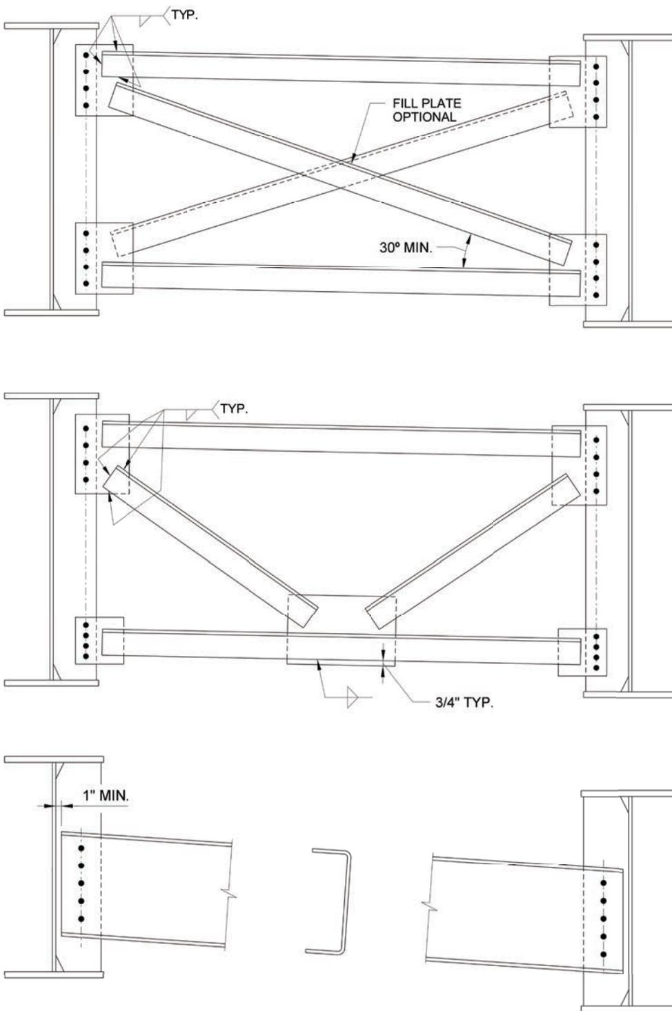
X-type cross-frame and K-type cross-frame bent-plate diaphragms (figures are from AASHTO/NSBA G12.1-2016).
