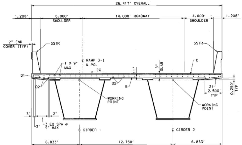
A sample twin-tub girder bridge cross section.
