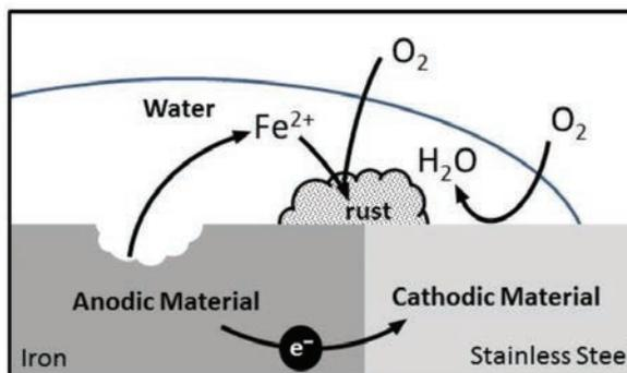
Fig. 1. An example of a galvanic cell.
