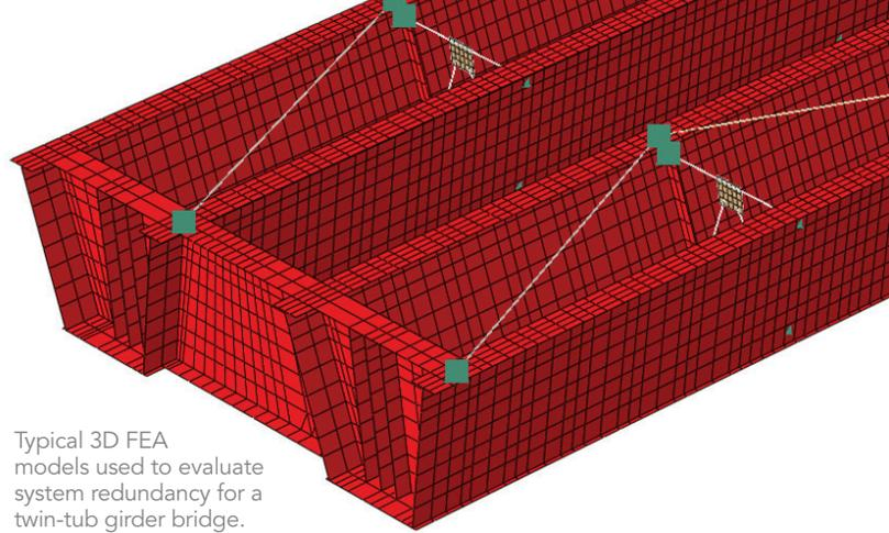
Typical 3D FEA models used to evaluate system redundancy for a twin-tub girder bridge.
