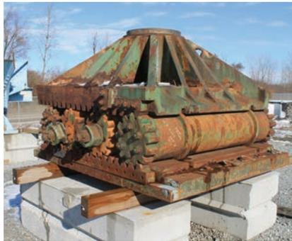
above: One of the more unique specimens at S-BRITE is this large nested roller bearing from one of the main river piers of the I-35W bridge.
