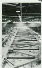
A 430' x 70' truss for a Burlington Northern railroad bridge being completely assembled in our shop.
