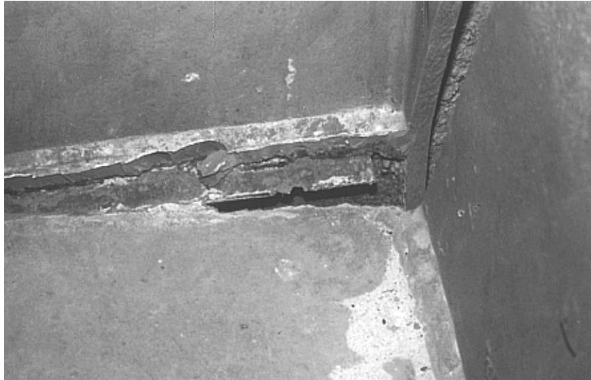
Figure 45 Lack-of-Fusion Defect Adjacent to Backing Bar at Gusset Stiffener Weld
