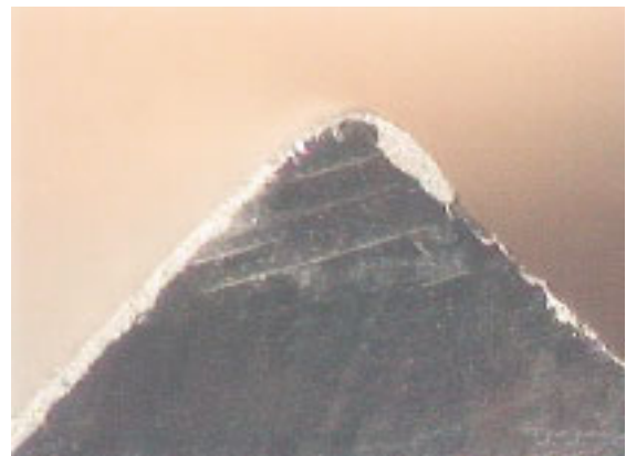
Phase 3, Photograph 66, Specimen 22 (organic [urethane] zinc) Corner MR-0 (90°)
