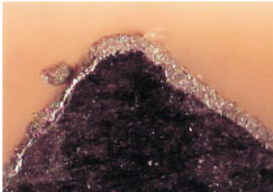
Phase 1, Photograph 14 Inorganic Zinc-Rich Primer (single coat) Corner MR-0 (90°)
