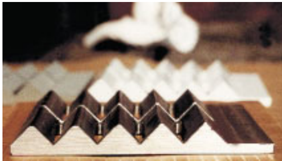
Phase 1, Photograph 2 Corner Grinding Test Specimen “As Fabricated Edge View”
