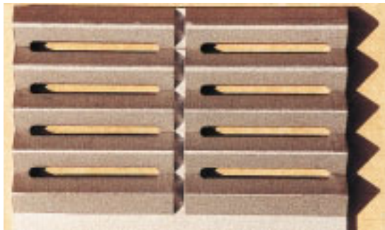
Phase 1, Photograph 3 Corner Grinding Test Specimen “As Fabricated and Blast Cleaned”
