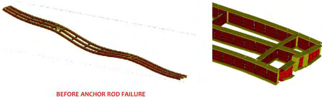
Figure 10: Deformed Structure at 4.2 \times \text{HL93} , prior to anchor rod failure (Deck not shown for clarity).
