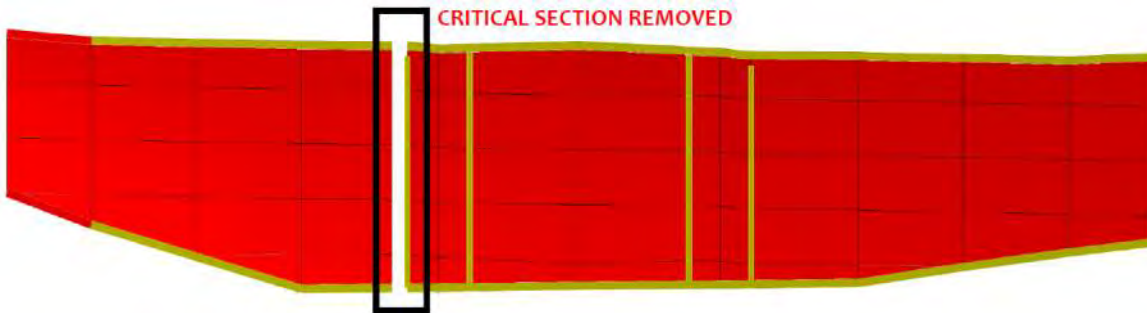
Figure 9: Damaged Condition of Pier Cap 11
