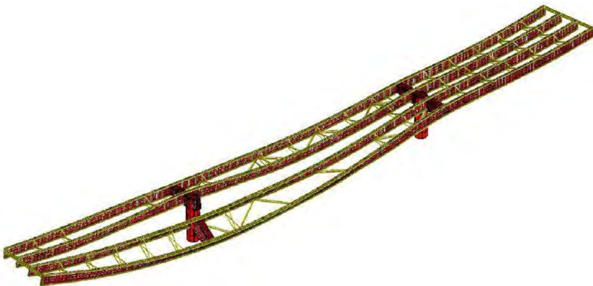
Figure 19: Framing plan after pier fracture near column, prior to live load (Deck not shown for clarity)
