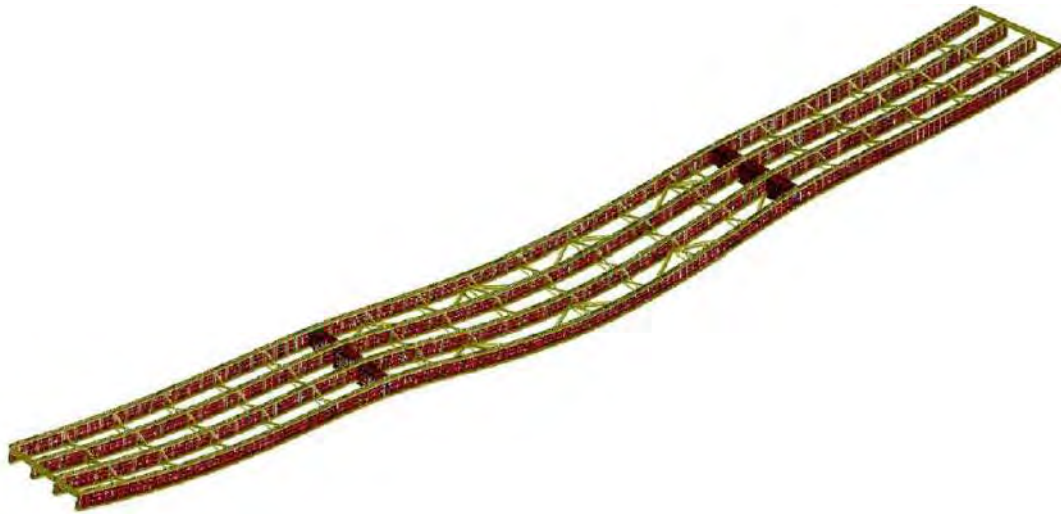
Figure 7: Deformed shape at 3.5 x HL-93 before hinging (Deck not shown for clarity)
