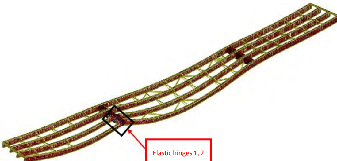
Figure 8: Deformed shape at 3.5 x HL-93 with elastic hinges at girders C and D (Deck not shown for clarity)
