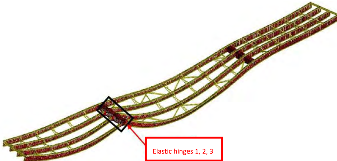
Figure 9: Deformed shape at 3.5 x HL-93 with elastic hinges at girders B, C, and D (Deck not shown for clarity)
