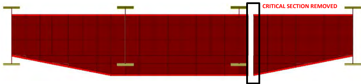
Figure 17: Location of Fracture in Damaged Condition at Integral Pier Cap Between Girders C and D
