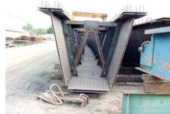
diaphragms and fewer girders versus plate girder alternates can speed erection, a critical advantage in urban highway reconstruction projects where traffic interruptions (and associated contractor “lane rental” penalties) dramatically affect construction costs and pose economic impacts to the community.
