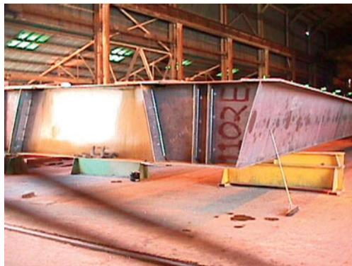
Figure 14: Full-depth plate girder sections are typically used for external end diaphragms. Access holes are sometimes required to facilitate field connection, but they were not used for this particular bridge.
