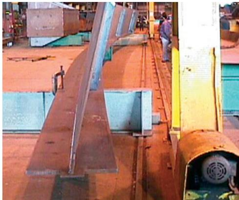
*Figure 20: Steel tub girders, top flanges and stiffeners are typically assembled as a sub-unit upside down, then flipped over and welded to the bottom flange.*
