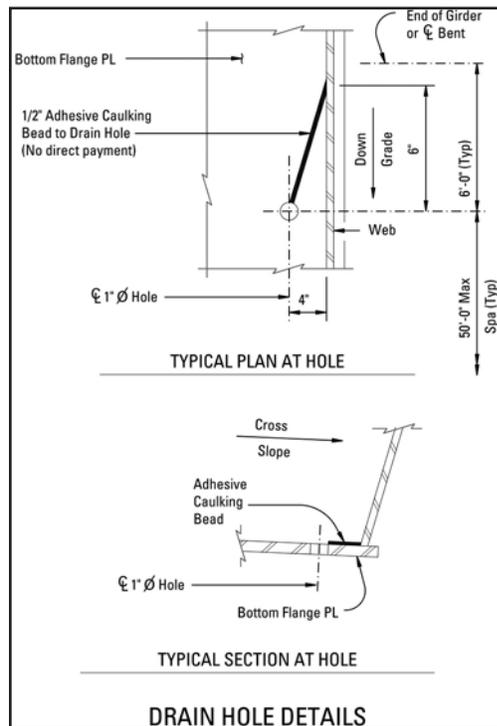
Figure 22: Suggested details for drain holes in tub girder bottom flanges.
