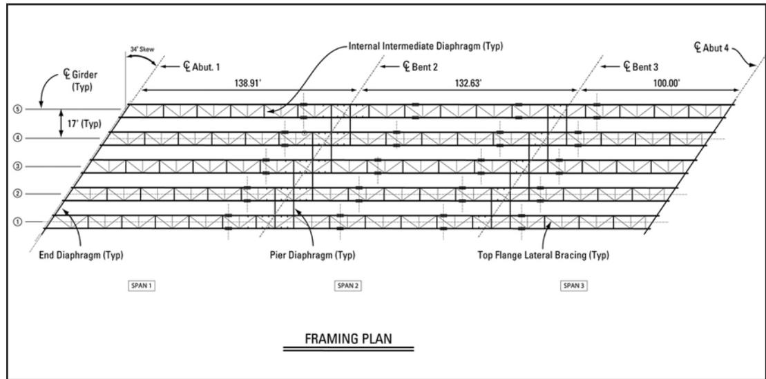
staggered, right (non-skewed) pier diaphragms to simplify detailing and erection. At the end diaphragms, there was not much choice but to detail the diaphragms on the 34-degree skew; the designers consulted a steel detailing shop and a local fabricator during the design process to solicit input on preferred details for the skewed end diaphragms.
