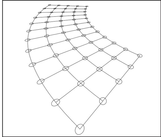
In a grid analysis, a two-dimensional grid is used to define the overall geometry, with line elements used to model the girders and diaphragms...
