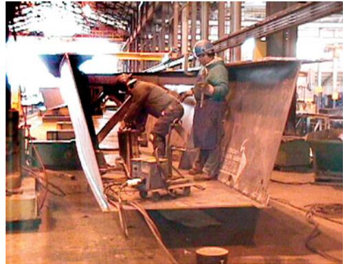
Figure 7: Maintain a minimum width of 4 feet for tub girders to allow room for workers to complete fabrication of various internal details.
