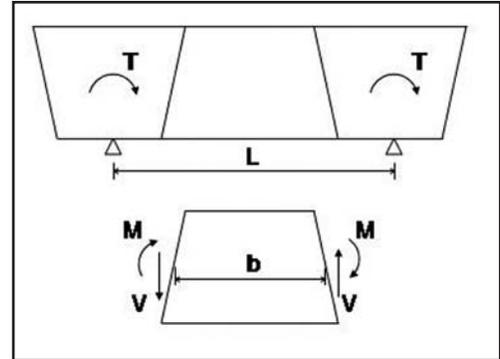
Figure 15: Freebody diagrams for calculating diaphragm forces.
