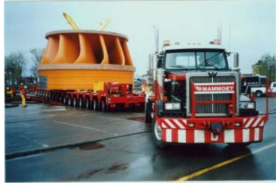
Pneumatic multi-axle trailer pulled by truck tractor.
