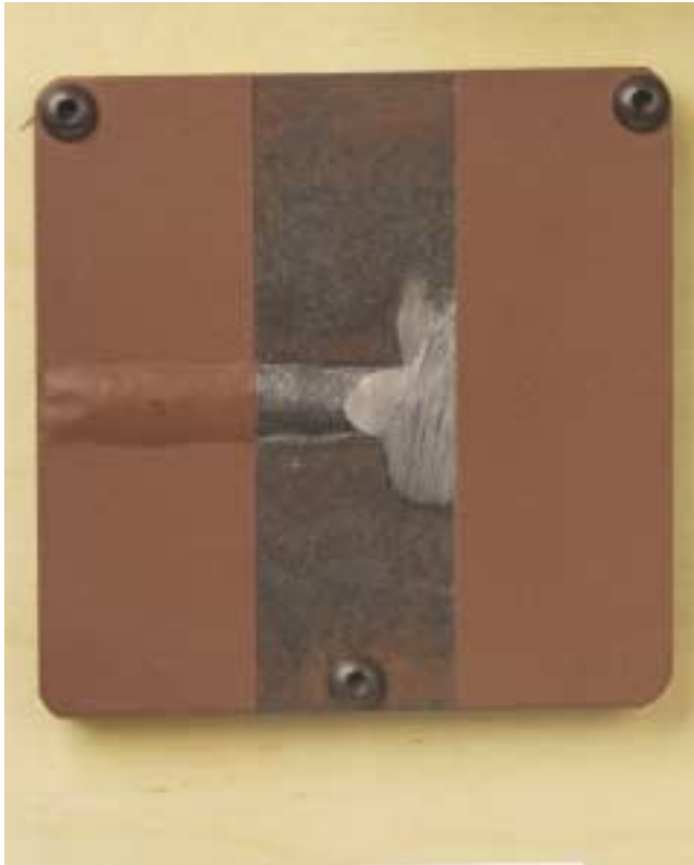
The left half of this sample shows a typical groove weld. The right half shows the same weld ground smooth.
