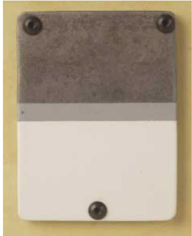
Interior environment, high-end primer/finish coating: epoxy finish coat with an epoxy or zinc rich primer, over an SSPC-3 surface preparation.
