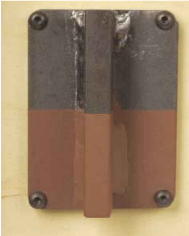
On the left, the fillet weld is continuous. On the right, the fillet weld is intermittent.
