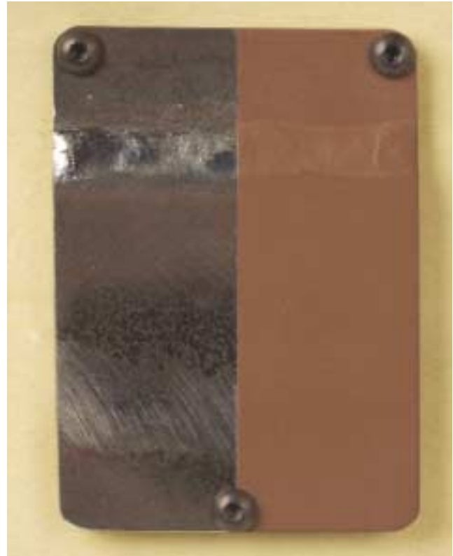
Weld show-through has been minimized.
