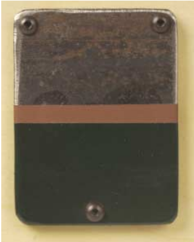
Interior environment, low-end primer/finish coating: alkyd (oil-based) finish coat with a shop-coat primer over an SSPC-3 surface preparation.
