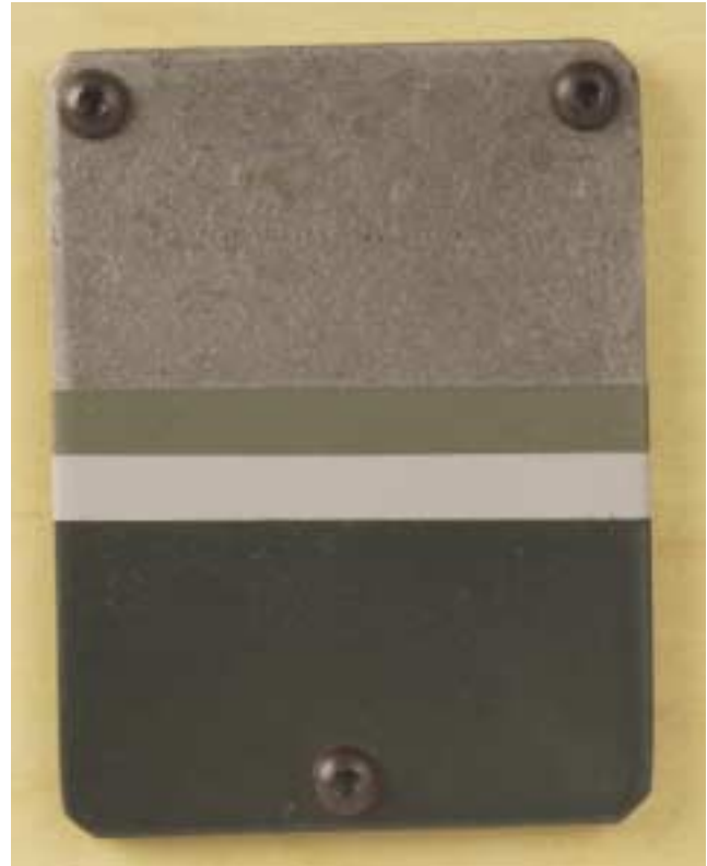
Exterior environment, high-end primer/finish coating: polyurethane finish coat with an epoxy intermediate coat and zinc rich primer over an SSPC-6 surface preparation.
