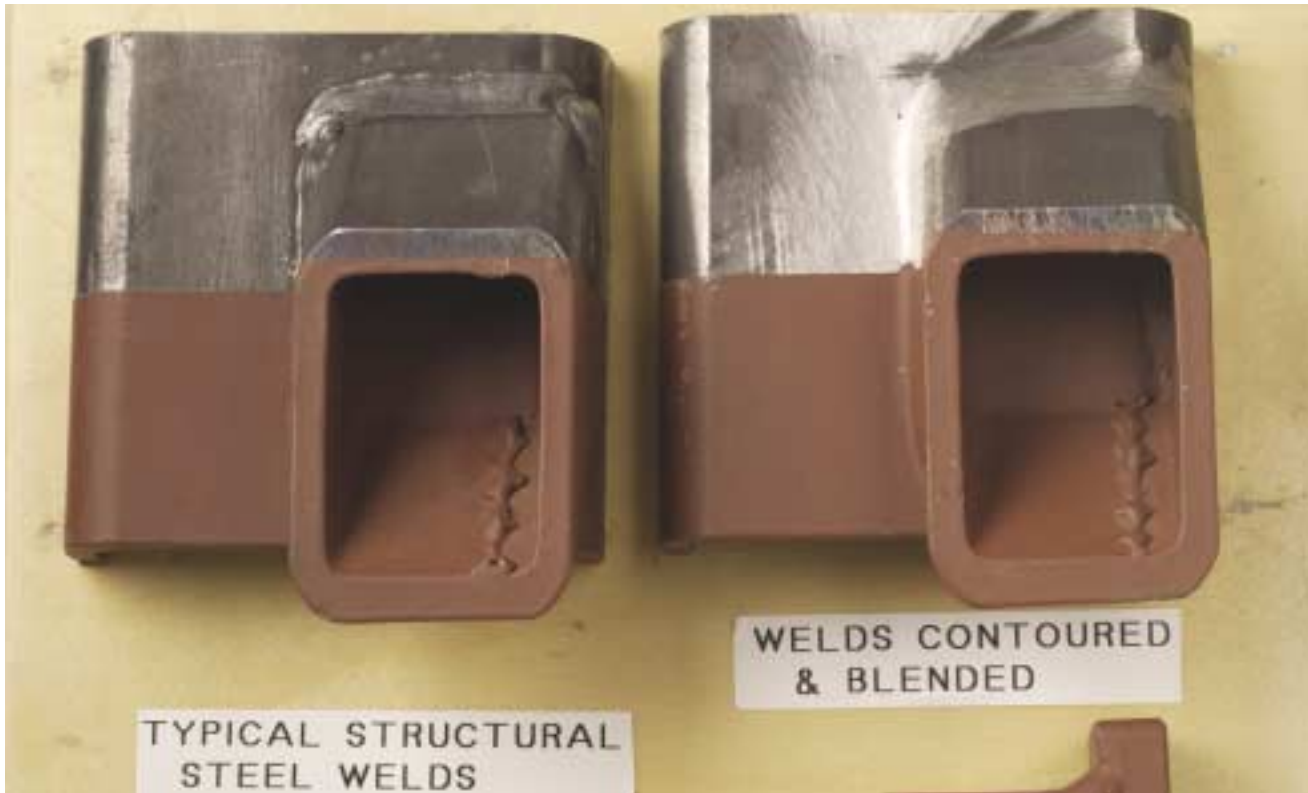
The sample on the left shows the appearance of typical structural welds. On the right, the welds have been ground smooth.
