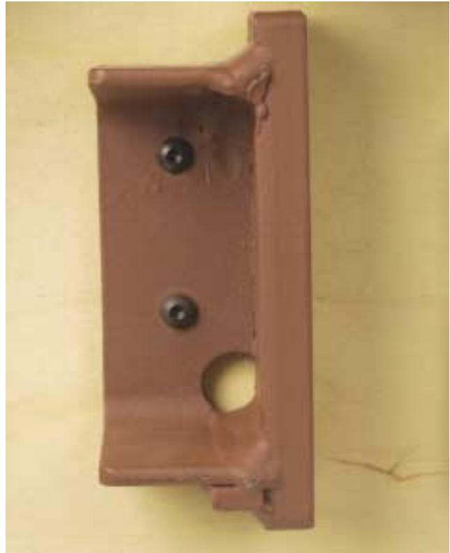
This sample shows atypical weld-access hole.
