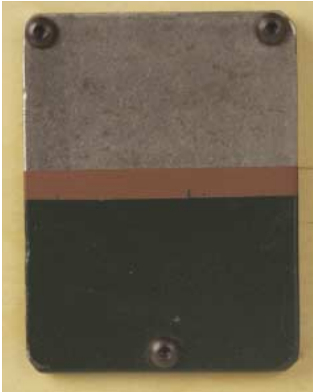
Exterior environment, low-end primer/finish coating: acrylic (water-based) finish coat with a shop coat primer over an SSPC-6 surface preparation.
