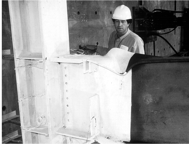
Figure 17 -. Extreme plastic deformation of beam-column connection designed for enhanced inelastic behavior
