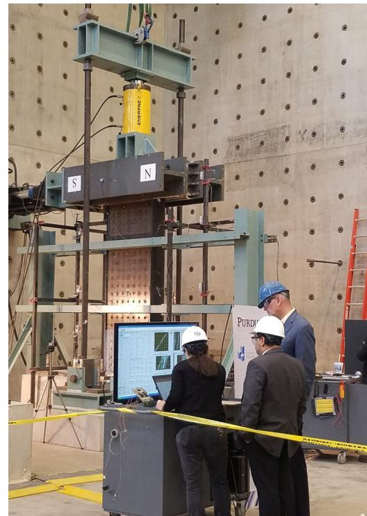
**GOOD RESULTS** Results of load tests to date have increased confidence in the core-wall system.
