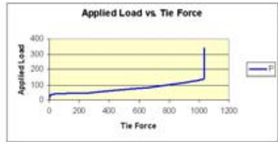
Figure-4: Relationship between applied load and catenary tie force
