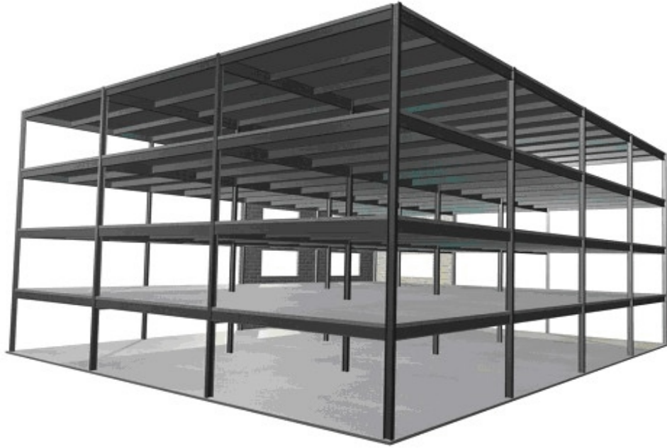
Figure 14 Proposed Full Scale Steel Test Building in the US (Mosher et al, 2001).
