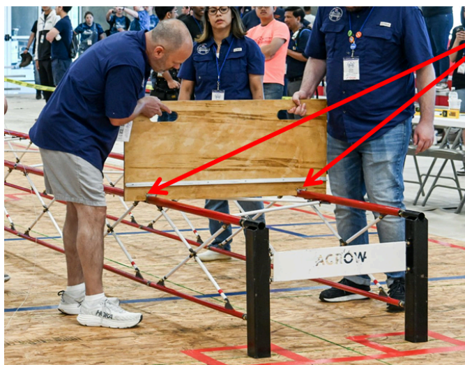
Figure 4: The top of the stringer must be in contact with the top of the two rabbets over the length of the stringers. The template shown is held plumb and perpendicular to the span of the bridge as it is slid down the length of the bridge. There should be no obstructions to its movement.
